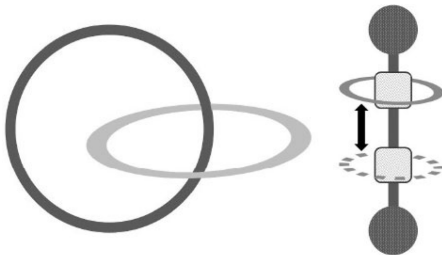
Figure 11-1: Catenanes (left) and rotaxanes (right) are made up of complex molecules that can be simplified in this schematic. (Left) Interlocked rings (silver and black) form from inter-ring attraction. (Right) A ring is threaded around a handle (solid black), which has two stable stations (patterned boxes). The capping dumbbells prevent the ring from slipping off. (Image by Joseph Meany.)
