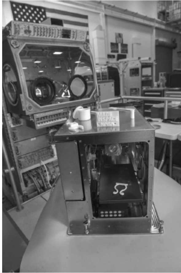
Figure 9-4: This first-generation, space-qualified 3-D printer, with the Microgravity Science Glovebox Engineering Unit in the background, was flown and tested in space aboard the International Space Station. (Image courtesy of NASA.)
