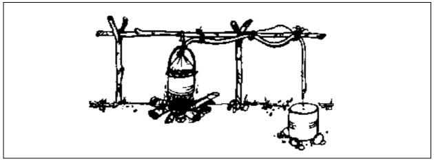
The condensation method of distilling water
