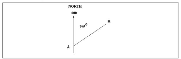
Measuring bearings in degrees [A - B = 045 degrees]
